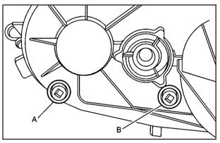
(A) Drain Plug (B) Filler Plug
